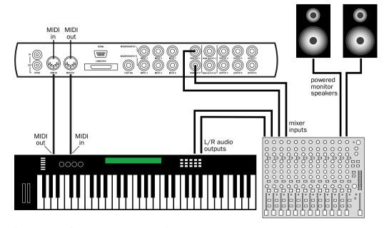
Basic MIDI setup using an external hardware mixer
