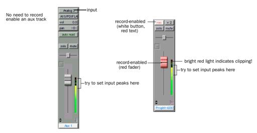
Setting recording input levels (Aux Track on left, Disk Track on right)
