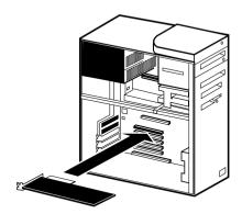
PCI card installation for an Intel computer
