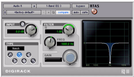
1 Band EQ set to Notch Filter
