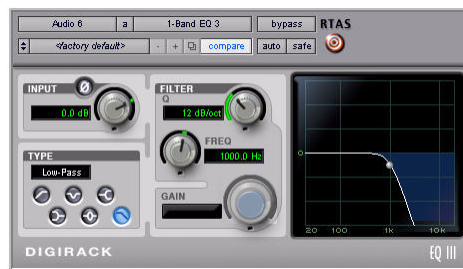
1 Band EQ set to Low-Pass Filter
