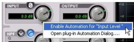
Enabling automation for a control
