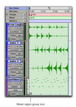
Mixed multitrack region group (sample- and tick-based audio, and tick-based MIDI)
