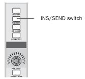
INS/SEND switch in a channel
