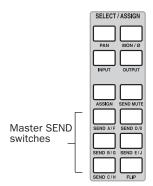
Master SEND switches in the SELECT/ASSIGN section
