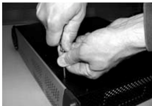
Removing the top cover screws
