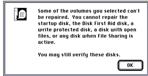
Figure 20. Disk Repair failure notification
