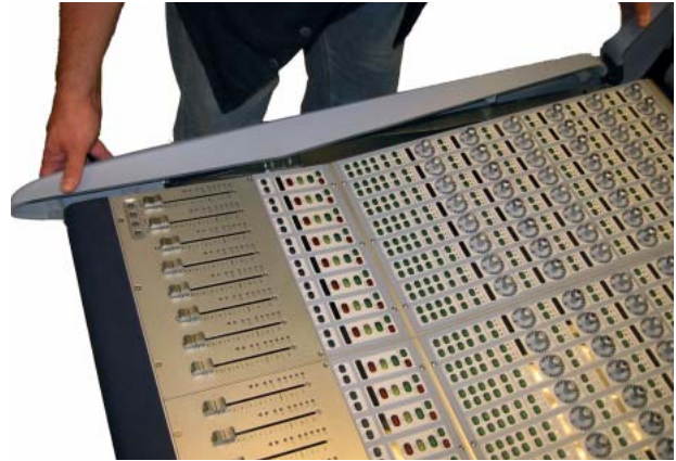
Figure 34. Placing a plastic side cap on the stand
