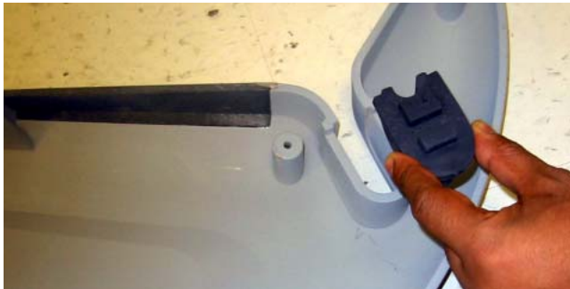
Figure 33. Installing a meter break cap in a plastic side cap
