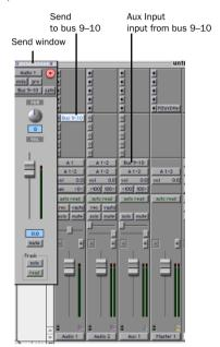
Audio and Auxiliary Input tracks configured for a send and return
