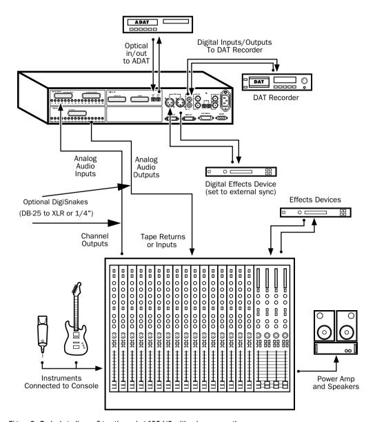
Figure 3. Typical studio configuration using 192 I/O with mixer connections
