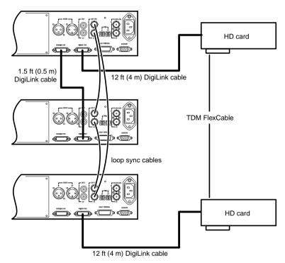
Figure 2. Three 96 I/Os, 48-channel
