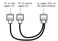
Optional 16-channel peripheral cable adapter
