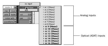
Figure 7. Routing an input to a mono track
