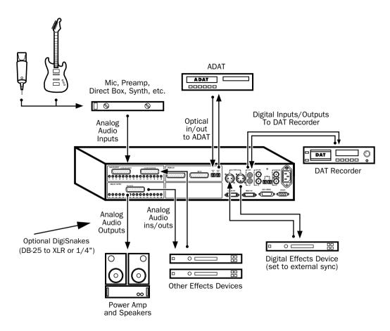
Figure 4. Typical studio configuration using 96 I/O without a mixer
