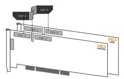
Inserting TDM FlexCable
