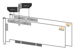
Inserting TDM FlexCable
