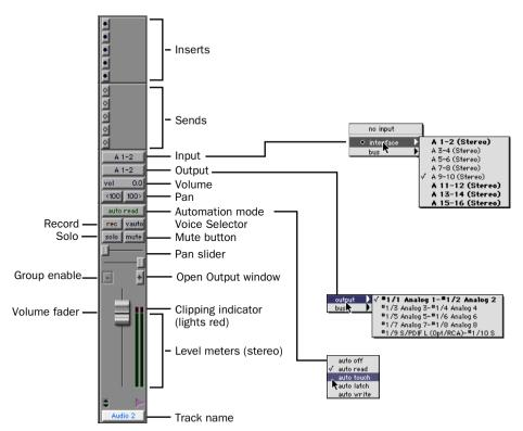
Figure 6. Stereo audio track in the Mix window
