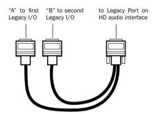
Optional 16-channel peripheral cable adapter
