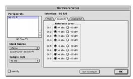
Hardware Setup, 96 I/O Analog In settings
