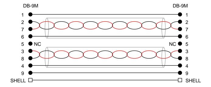
All Pins Wired Straight Through Pins 2 & 7 are a Twisted Pair with Shield Drain Wire on Pin 6 Pins 3 & 8 are a Twisted Pair with Shield Drain Wire on Pin 4 This is a standard ESBus Machine Control Cable
