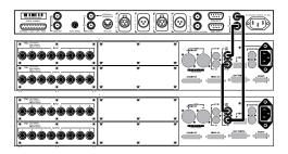
Loop Sync in an expanded Pro Tools | HD system
