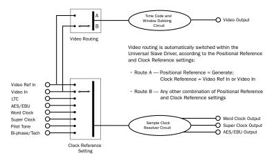
Figure 1. Video Input Flow diagram
