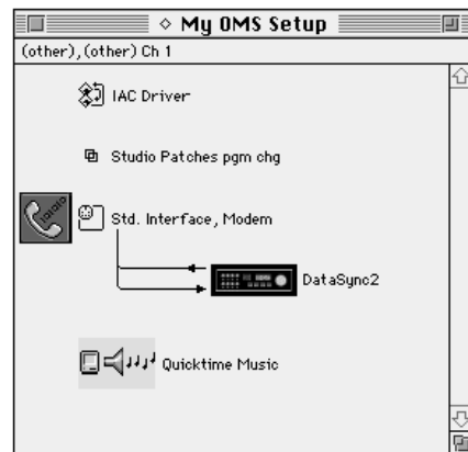
Connecting a peripheral (in this case, a DataSync2) to the correct port in the OMS Setup window
