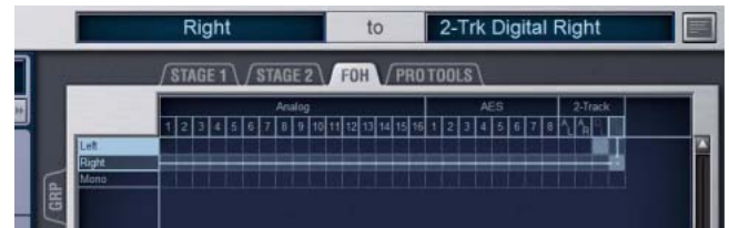
Routing 2-Track output in the Patchbay
