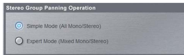
Setting the Group bus operational mode
