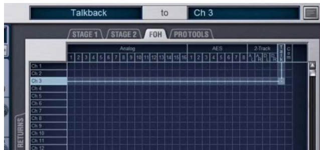
Routing Talkback input in the Patchbay
