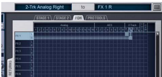
Routing 2-Track input in the Patchbay
