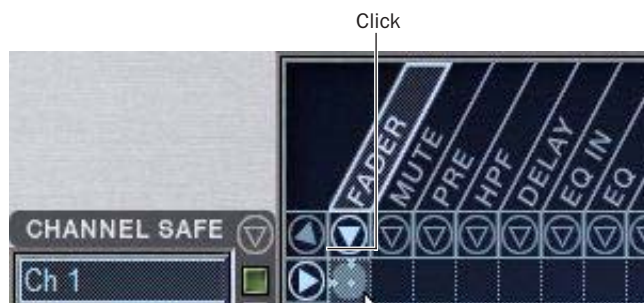
Enabling recall safe for channel 1 fader
