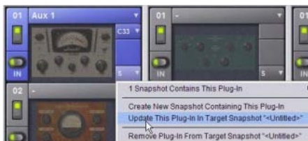
Updating plug-in data in an associated snapshot from the plug-in view
