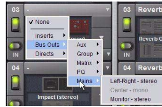
Assigning monitor output to a bus-fed plug-in
