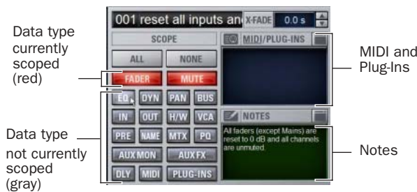
Data Type Scope buttons showing different scope states
