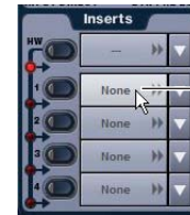
Assigning a plug-in insert in the Inputs page
