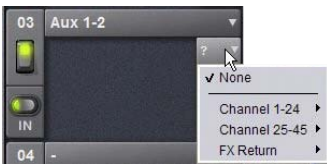
Assigning plug-in output to an FX Return
