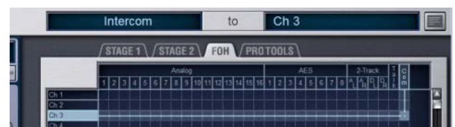
Routing Intercom input in the Patchbay
