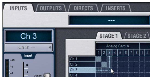
Assigning an input source in the Patchbay Inputs page
