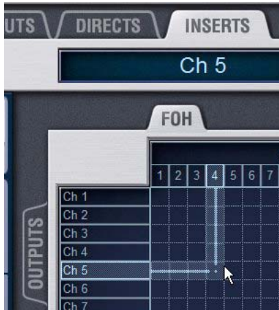
Assigning a hardware insert in the Patchbay Inserts page
