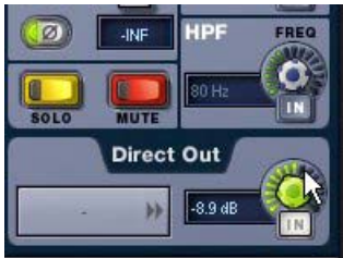
Adjusting Direct Output level from the Patchbay
