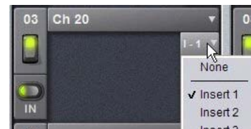
Channel Insert selector for a plug-in rack
