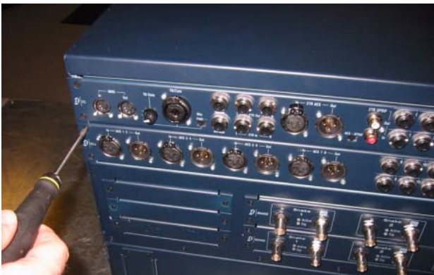
Securing the IOx card to the back panel of the FOH Rack
