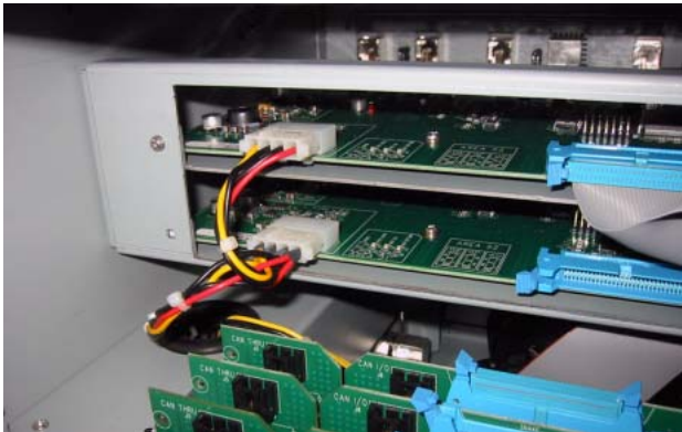
Power connection to the Snake card
