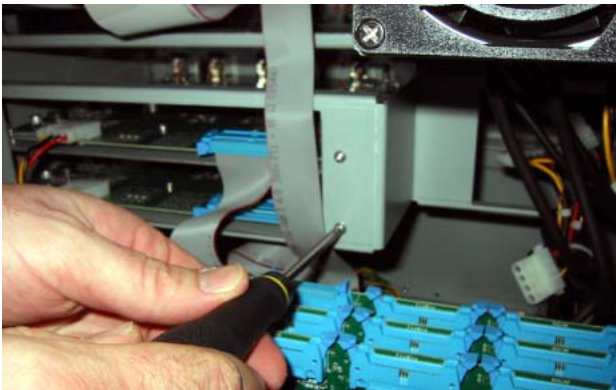
Securing the Snake card to the FOH Rack chassis
