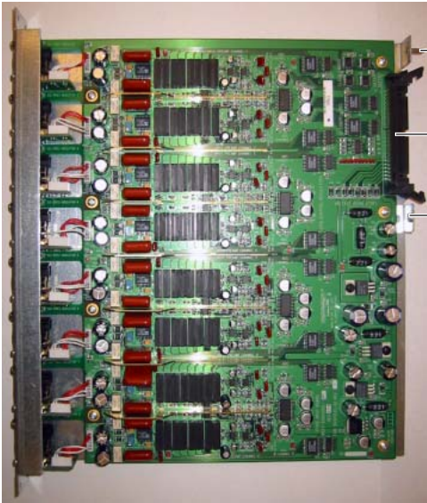
Stage Rack I/O card showing brackets and connector
