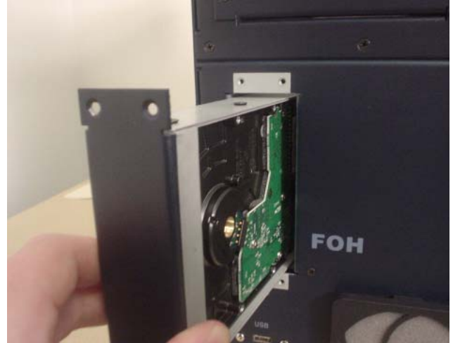
Sliding the hard drive bay from the FOH Rack
