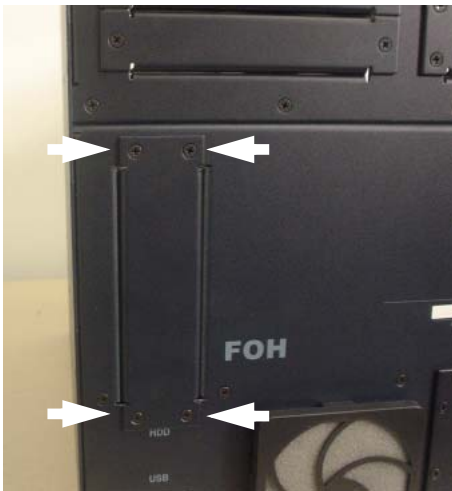
Removing the hard drive bay from the FOH Rack
