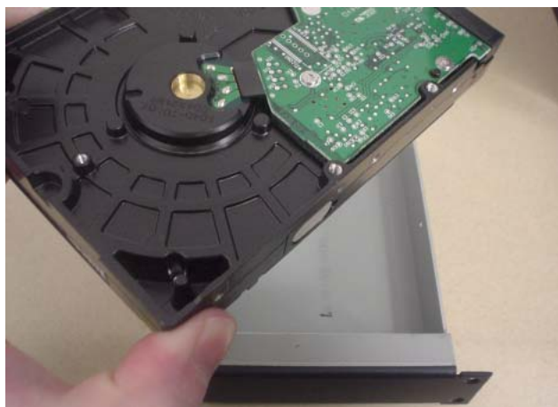
Lifting the hard drive from the drive bay
