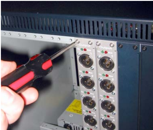
Securing a Stage Rack I/O card to the Stage Rack front panel
