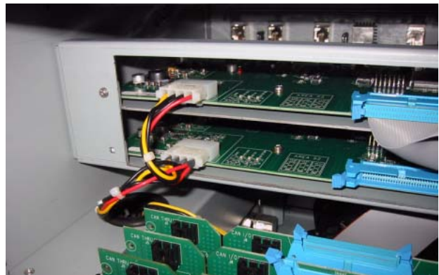
Power connection to the Snake card
