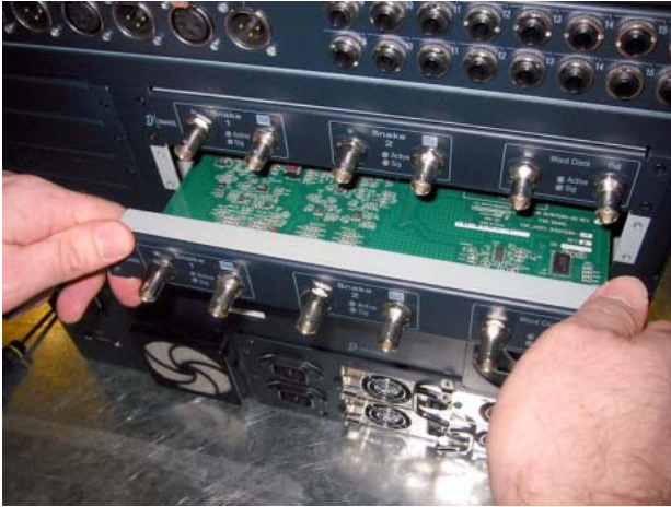
Installing the Snake card in the FOH Rack
