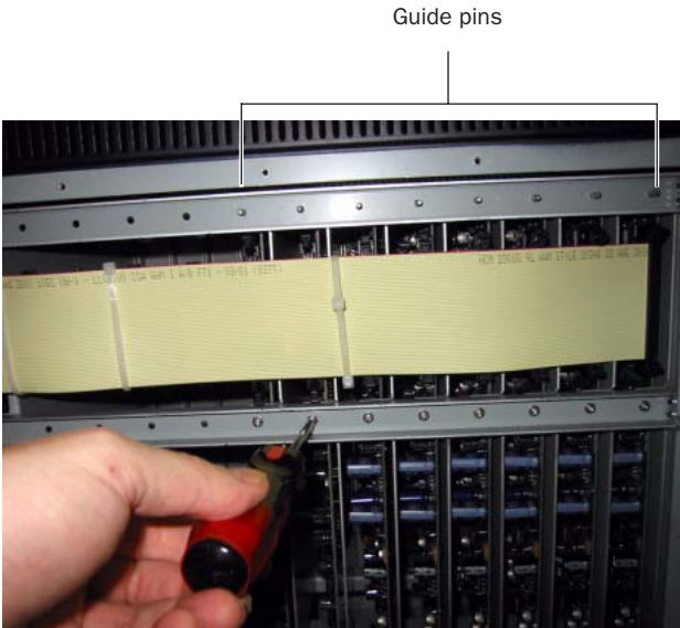
Securing a Stage Rack I/O card to the Stage Rack chassis
