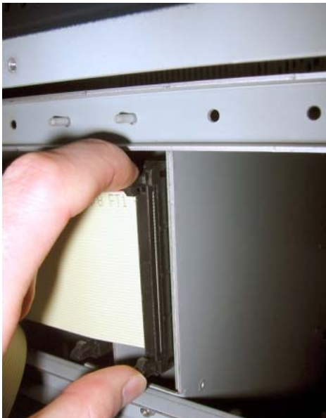
Connecting a Stage Rack I/O card to the Stage Rack ribbon cable
