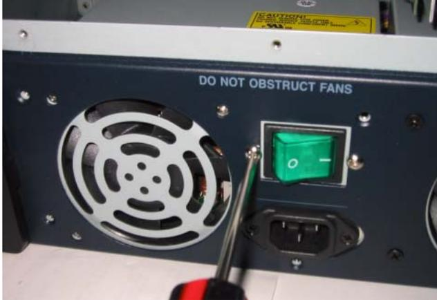
*Securing the power module to the chassis*
