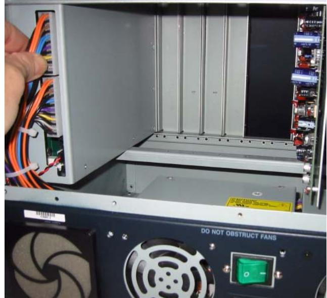
*Connecting the new power module to the Stage Rack*
