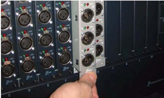
*Removing a Stage Output card from slot G*
