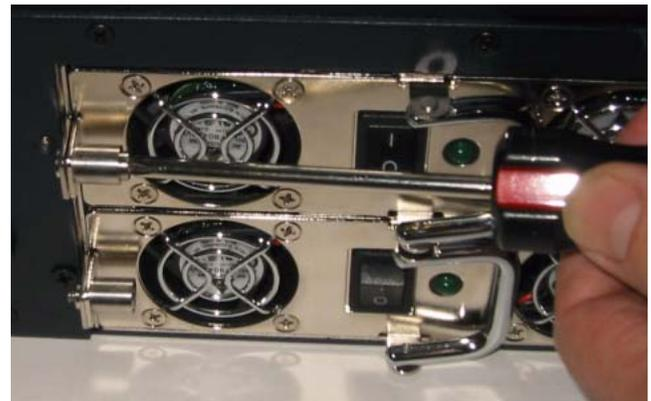
*Securing the mounting screw to the chassis*
