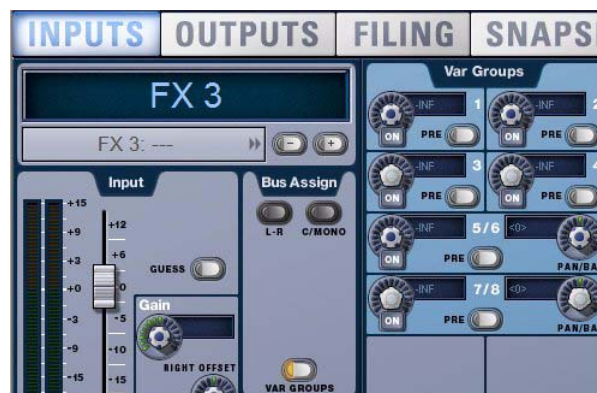
Variable Group controls displayed in the Inputs page
