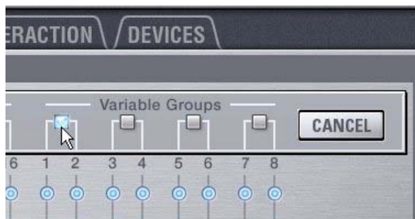
Linking a Variable Group bus pair
