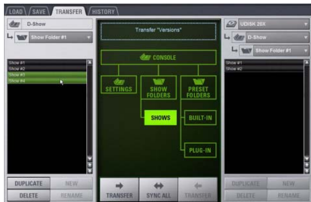
Show files selected for transfer from D-Show to USB key disk
