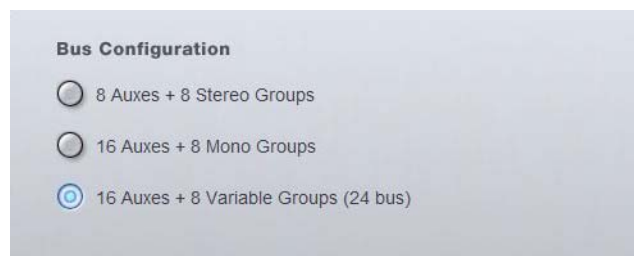
Selecting the Variable Groups bus configuration
