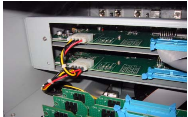
Power connection to the Snake card
